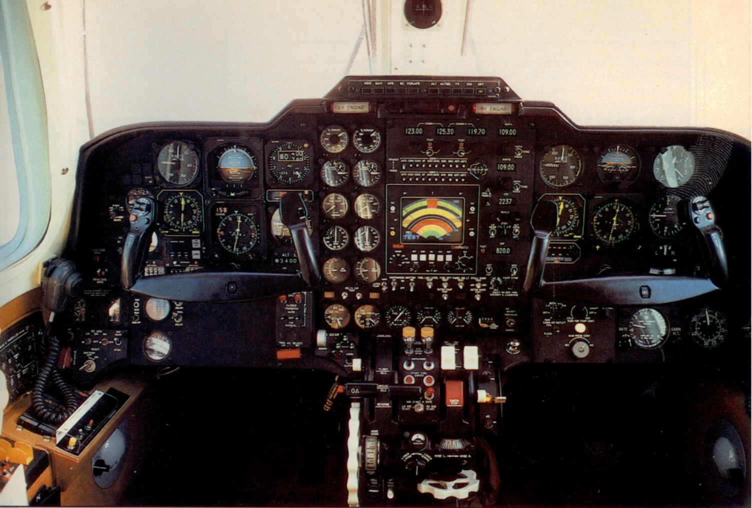
Much of the equipment in the MU-2's well-equipped cockpit is standard, including a Sperry autopilot/flight-director system. A known-icing package is also standard. Passengers are well accommodated, too.
